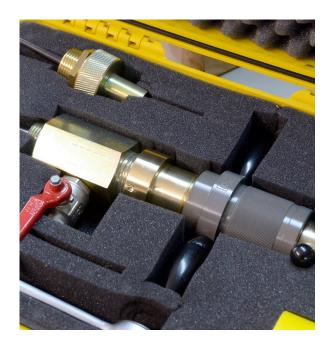
The hot tap drill is the universal tool to install your insertion flow meter in any compressed air system. In only 30 minutes you can drill a hole and install your flow meter. Using a hot tap saddle and a hot tap drill, you can create a new installation point without depressurizing your installation. Compared to low-cost electrical hot tap drills, which are prone to jamming and breaking of the drill head, our hot tap drill is safe and easy to operate.
